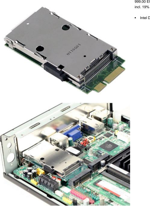
All Intel DN2800MT or Mitac PD10BI boards have a cutout slot for inserting 34mm Express Card.
